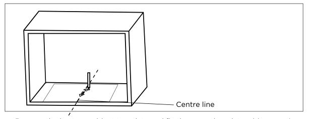
• Remove the bottom cabinet template and fix the mounting plate with screw A.
