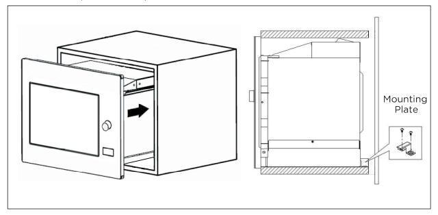
• Open the door, fix the oven to the cabinet with Screw B, at the installation hole. Then fix the Trim-kit plastic cover to the installation hole.
